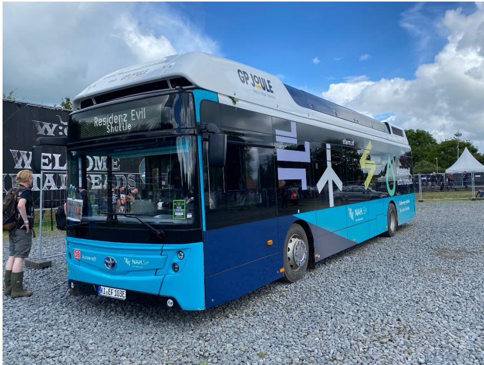
Caption 2: CO2-free to the Holy Ground - the hydrogen-powered eFarm bus is used for shuttle services around the festival.
